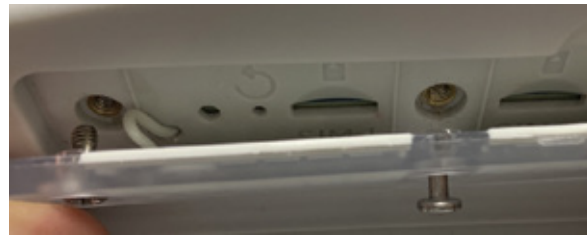
Incorrect tether placement
